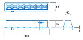
Cut out : 49mm x 288mm Void depth : ≥120mm
