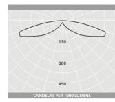
AREA DISTRIBUTION Luminaire Lumen Output: 3000K 11W = 735lm 21W = 1255lm 4000K 11W = 875lm 21W = 1495lm
