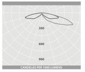
PATHWAY DISTRIBUTION Luminaire Lumen Output: 3000K 5W = 380lm 11W = 655lm 4000K 5W = 450lm 11W = 780lm
