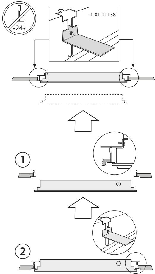
**B. MOUNTING** - Montage - Installation - Montaggio - Montering
