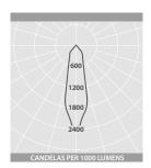
**NARROW BEAM** Luminaire Lumen Output: 2W = 260lm
