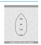
**WIDE BEAM** Luminaire Lumen Output: 2W = 260lm
