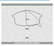
ROADWAY DISTRIBUTION Luminaire Lumen Output: 31W = 4225lm 48W = 6890lm
