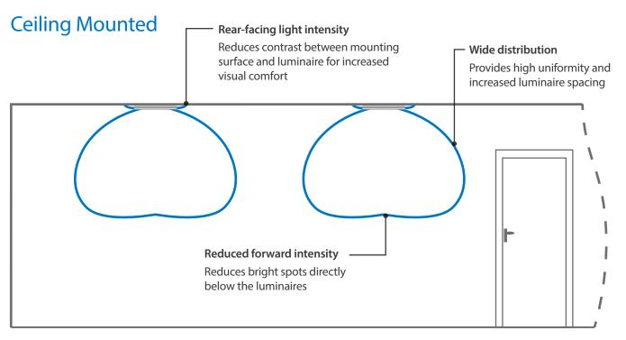
The high performance reflector produces a broad light distribution, excellent for wide luminaire spacing and provides high uniformity. The distribution of light is ideal for corridors and stairwells when either wall or ceiling mounted.
