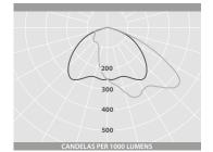
Luminaire Lumen Output: 52W = 6360lm 78W = 9155lm DIMENSIONS
