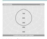
Luminaire Lumen Output: 98W = 16555 lm 137W = 22410 lm
