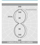
Luminaire Lumen Output 10W = 1560lm 20W = 3095lm
