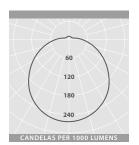
Luminaire Lumen Output: 8W = 1290lm 16W = 2385lm 20W = 2990lm 26W = 3945lm
