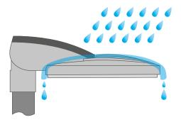
"Free draining" curved heat sink eliminates ponding of fluids 2
