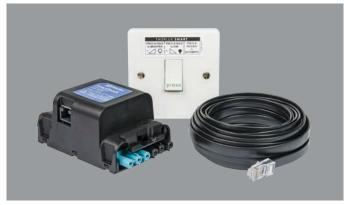
Any number of retractive switches can be connected to the Motionline to provide group dimming control of Smart luminaires. In normal operation each Smart luminaire will automatically adjust its own luminance level to maintain the preset required light level. When controlled via the switch all the luminaires will initially synchronise to the same lighting level which can then be varied from 100% to 1% (some ballasts are limited to 10%) and off.
