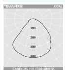
BROAD DISTRIBUTION Luminaire Lumen Output: 22W = 3920lm 30W = 5355lm 52W = 9115lm
