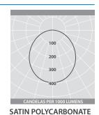
Luminaire Lumen Output 8W = 730lm 16W = 1460lm
