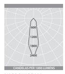
**NARROW BEAM** Luminaire Lumen Output: 2W = 260lm
