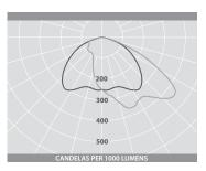
Luminaire Lumen Output: 52W = 6360lm 78W = 9155lm
