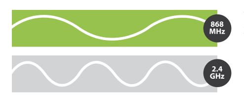
Operational frequency 868MHz - relatively long wavelength compared to common 2.4GHz systems – provides greater distance and penetration of signals.
