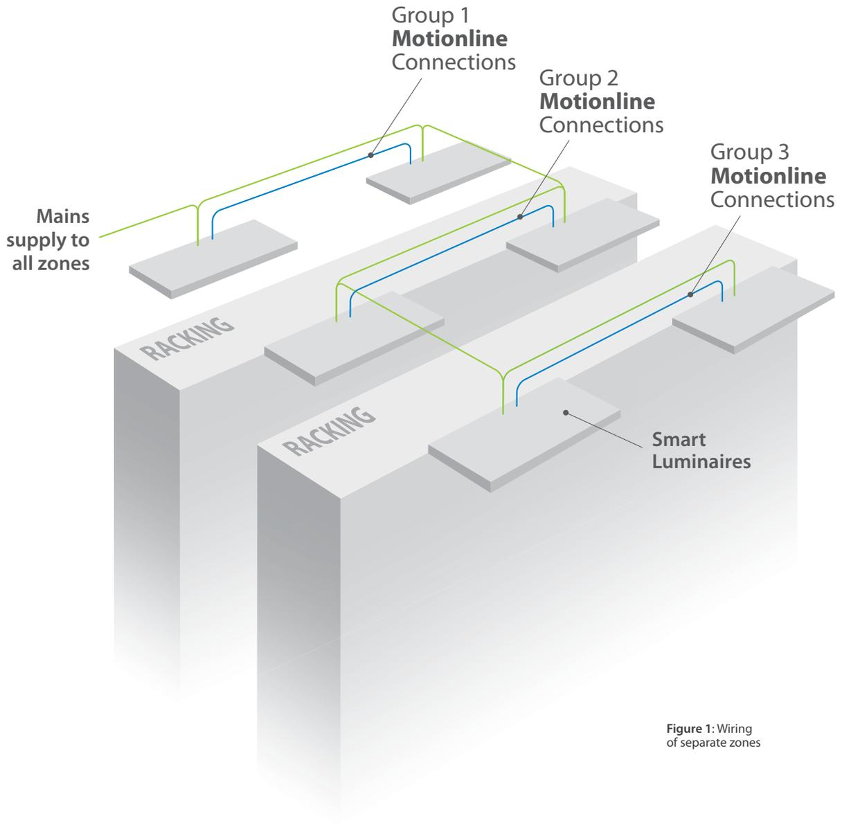
Figure 1: Wiring of separate zones
