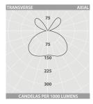
Luminaire Lumen Output: 10W = 1665lm 17W = 2705lm 24W = 3685Im
