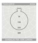
CLOUD 4 Luminaire Lumen Output: 29W = 4170lm 30W = 4170lm
