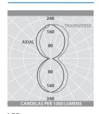
LED Luminaire Lumen Output 10W = 1430lm 20W = 2640lm
