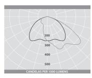
Luminaire Lumen Output: 52W = 6360lm 78W = 9155lm
