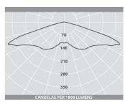
Luminaire Lumen Output: 30W = 3975lm 60W = 7340lm
