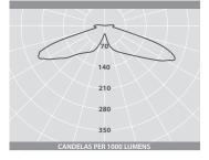
Luminaire Lumen Output: 31W = 4320lm 52W = 6825lm
