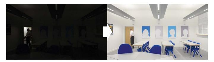
When you enter the room the first light will detect you and tell the other lights to turn on. The lights will remain on while the space is occupied, every light has a sensor that will see the slightest hand movement, so don't worry, the lights will never turn off when you are in the room. When you leave the room the lights will wait ten minutes and then turn off (10 minutes is the standard setting but can be changed).
