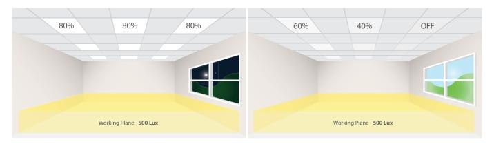
A completely "free" source of light is the sun, the Smart system knows this and takes full advantage. Each light is set to maintain an exact lighting level on the working surface (desk etc.), if daylight enters the space then the lights will dim automatically to compensate for this, saving energy. In areas with large amounts of daylight the lights may switch off completely.
