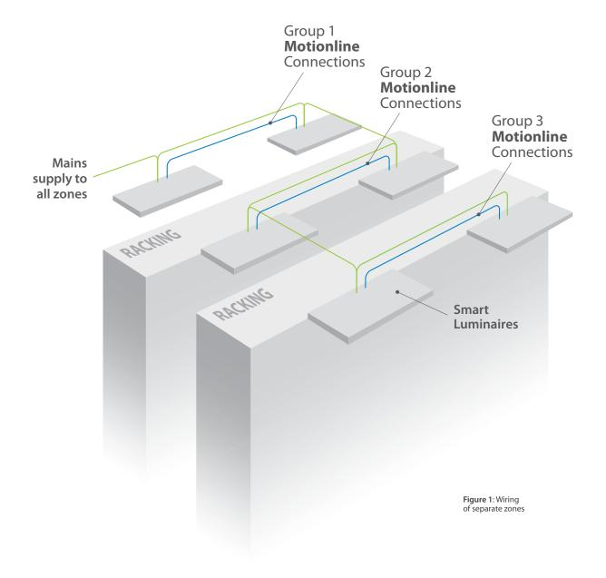
Individual Thorlux Smart luminaires may be linked into a grouped system using a "Motionline" two wire low voltage bus allowing luminaires to communicate within a group
